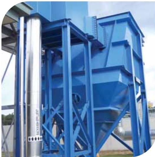
The clarified liquid leaves the plate assembly through orifices or weirs at the top and is distributed into collection channels leading to the clarified water outlet. This creates a pressure drop across the collection channels which ensure uniform flow distribution across the plates in order to utilize the full area for settling.
